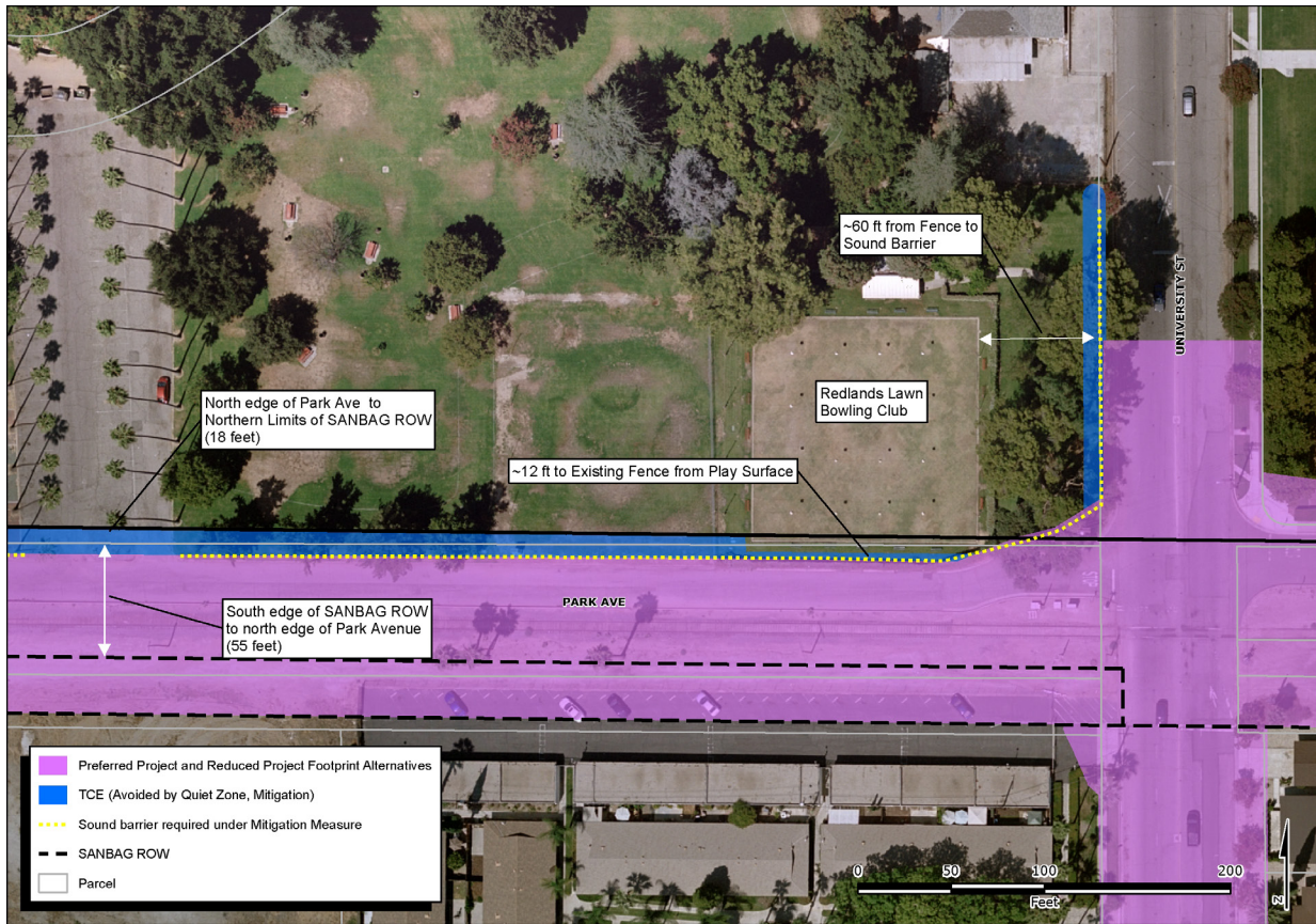
Figure 5-11. Sound Barrier Locations with Distances between Barrier Segments and Redlands Lawn Bowling Club Green.
