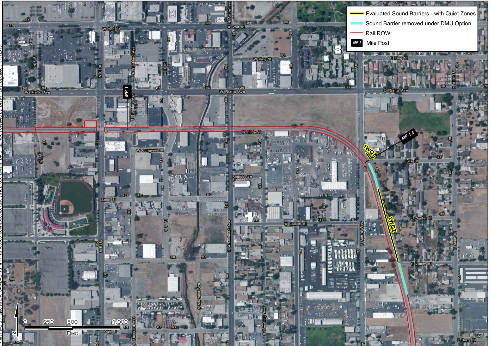
Evaluated Sound Barrier Locations Under DMU Option - Scenario with Implementation of Quiet Zones
