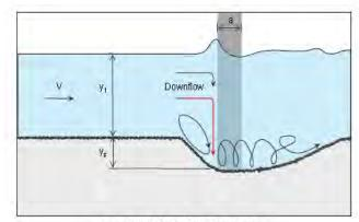
$$\frac{y_a}{a_d^*} = 2.0 \text{ K}_1 \text{ K}_2 \text{ K}_3 \left(\frac{y_1}{a_d^*}\right)^{0.35} \text{ Fr}_1^{0.43}$$
