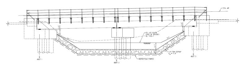
ELEVATION - BR 9.4 ABUTMENT AND CHANNEL PROTECTION NO SCALE
