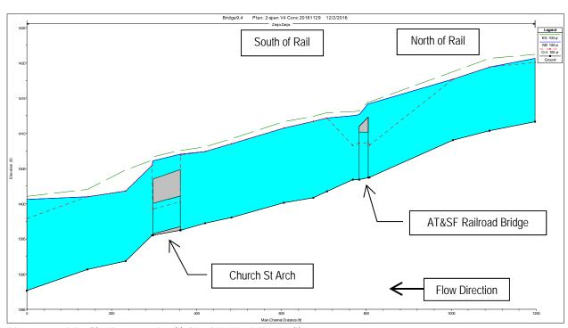
EG = energy grade line (ft), WS = water surface (ft), Crit = Critical Depth Elevation (ft), yr = year
