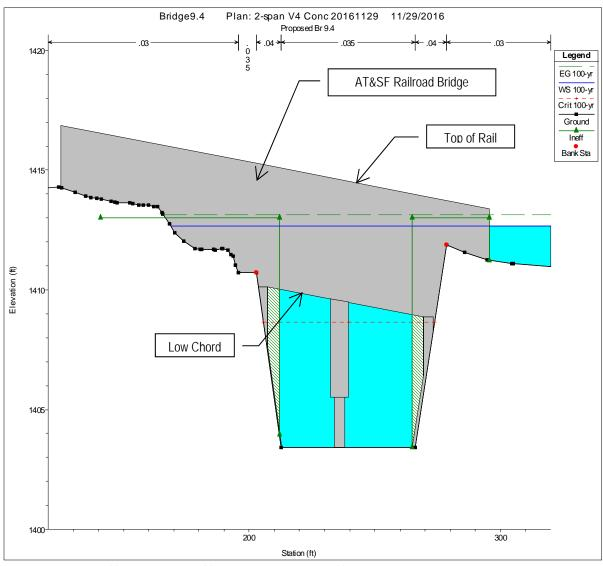
EG = energy grade line (ft), WS = water surface (ft), Crit = Critical Depth Elevation (ft), yr = year, Ineff = Ineffective Flow Area, Sta. = Station
