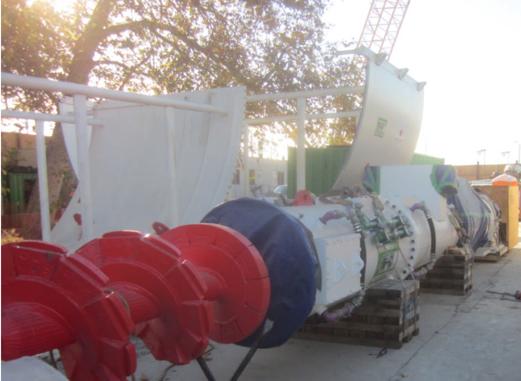
Tunnel Boring Machine Screw Conveyor.
