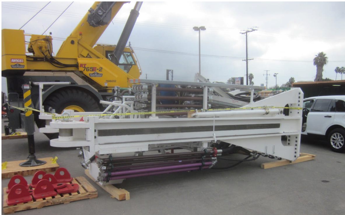
Tunnel Boring Machine Erector Main Beam.
