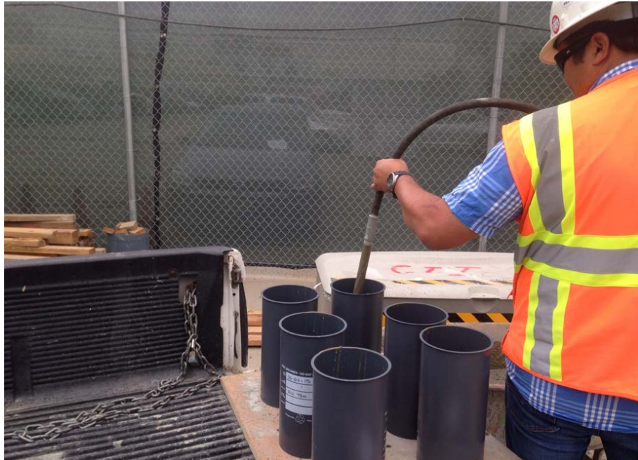
C0980 – RCC QC taking concrete test at Mangrove location
