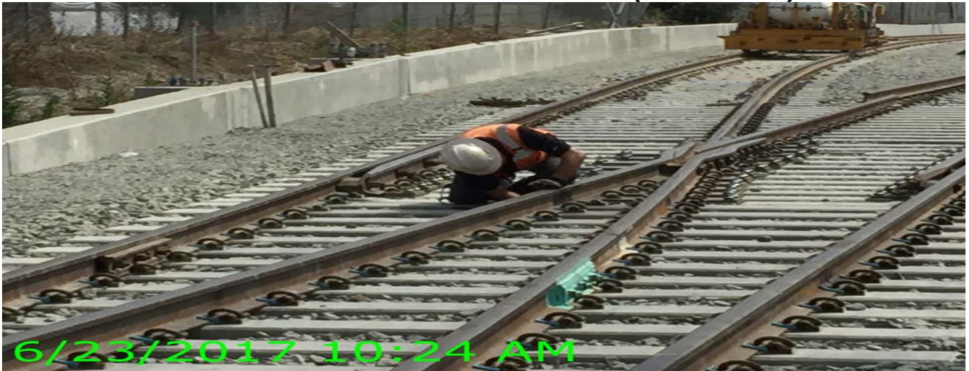
B1 GUIDEWAY – Herzog performing hand held UT testing between Centinela and High St.
