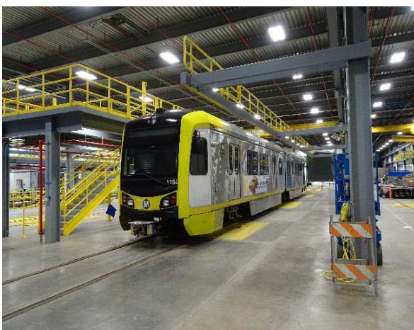
Division 16 - train on heavy repair platform in main shop
