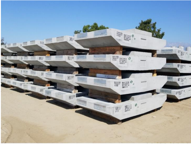
Pre-fabricated Floating Slabs ready for delivery
