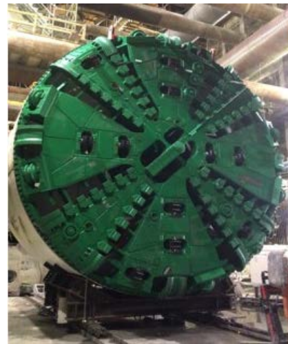
TBM Assembly at the Launch Box in Century City
