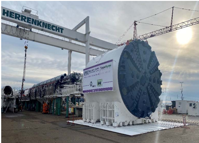
Tunnel Boring Machine
