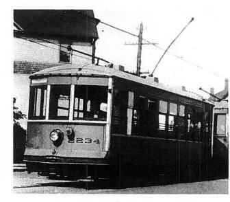
The Birney "Safety" Car permitted a single operator to perform the duties formerly requiring both a motorman and a conductor. Transit systems large and small, including The Connecticut Company pictured here, assigned four-wheel (single-truck) Birneys to lightly patronized routes. But if you think the cable car was used only on hills, you're wrong. San Francisco had the most trackage, but the heaviest traffic and most cars were in Chicago, where hills aren't that much of a problem.
