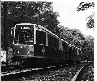
The two Standard Light Rail Vehicles in this **Massachusetts Bay** Transportation Authority train are among the first light rail cars manufactured in the United States since 1952, Each two-section articulated vehicle carries up to 219 passengers, has a maximum speed of 50 mph. and can be coupled into multiple-unit trains (as shown). These SLRVs replace aging Electric Rallway Presidents' **Conference Committee** (PCC) cars on the MBTA private right-of-way Green Line.
