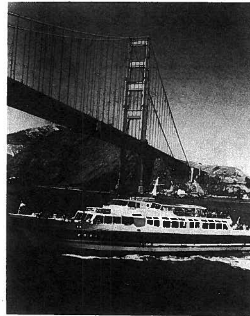
Transit systems operate a wide variety of passenger vehicle types. Pictured here are one of the largest and one of the smallest U.S. transit vehicles. This Hop-a-Bus (above), operated in downtown loop service by the Dallas Transit System, is 21 feet long and carries 19 passengers whereas the Golden Gate Transit ferry boat Marlin (left) is 165 feet long and carries 750 passengers.
