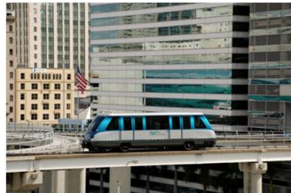
Automated Guideway Transit trains provide distributor or shuttle service without an on-board operator, offering the potential for lower operating costs. The Miami-Dade Transit Metromover has 21 stations in downtown Miami and adjacent neighborhoods. Connecting major buildings and transportation access points, the Metromover is considered to be an important factor for downtown development in Miami. Automated Guideway Transit modal data are included with other rail modes on on Tables 27 and 31.
