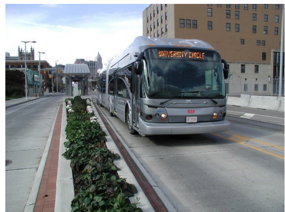
The Greater Cleveland Regional Transit Authority Health Line provides bus rapid transit service in bus-only lanes that are prohibited to other vehicles. This BRT bus is headed east on Euclid Avenue toward University Circle from downtown Cleveland, OH. Bus rapid transit data are reported in Tables 29 and 31.
