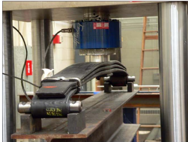
Figure 14. Laboratory test of a Freightliner FLD120 Tractor front suspension leaf spring
