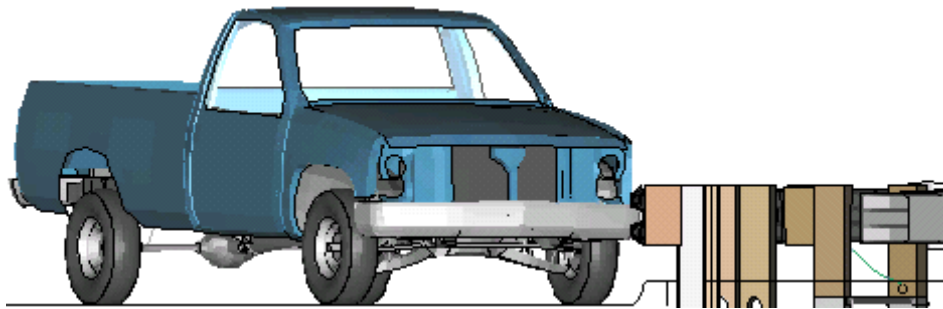
Figure 64. Finite element model for the analysis of the G4(1S) and AASHTO B curb. (146)
