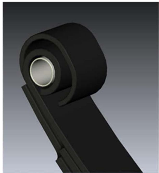
Figure 88. Digitized three dimensional geometry of the 1992 Freightliner FLD 120 suspension (Case 4).
