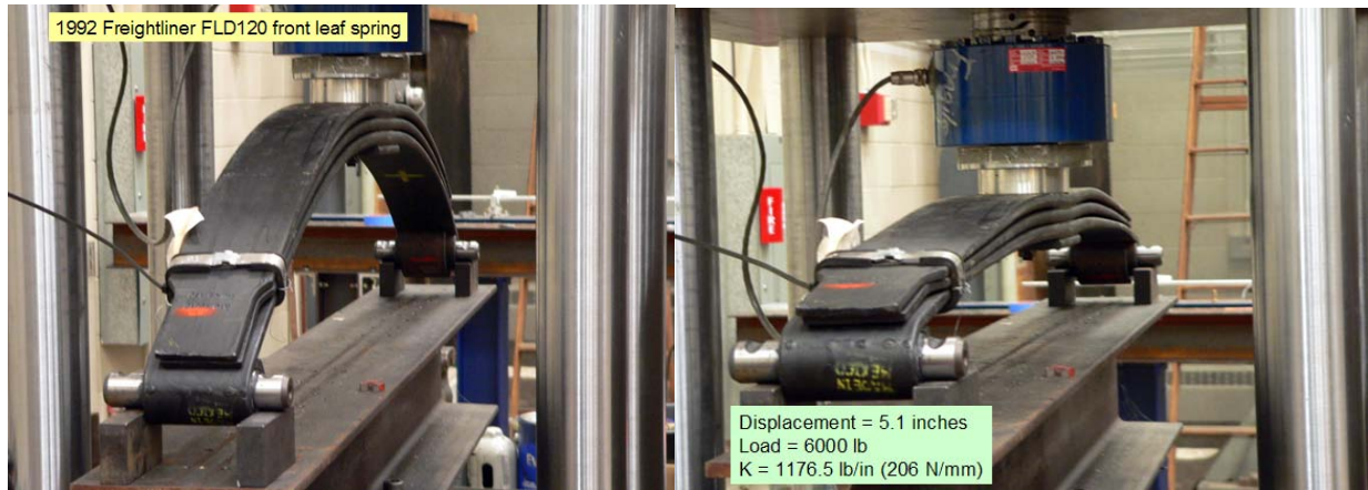
Figure 87. Laboratory Test of a 1992 Freightliner FLD120 Leaf-spring Suspension (Case 4).
