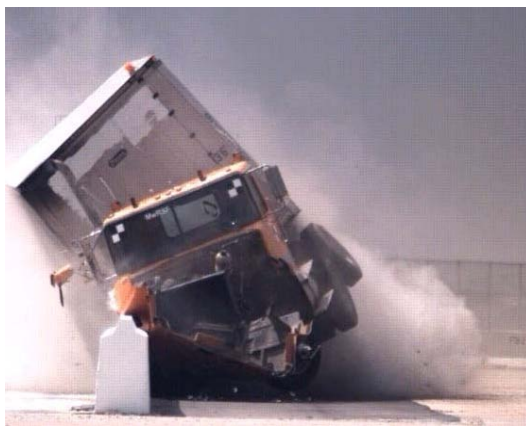
Figure 93. Summary of Phenomenological Events that Occurred during Full-scale Test and Finite Element Model Simulation in Case 4.
