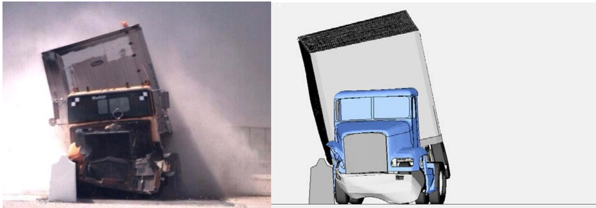
Figure 93. Summary of Phenomenological Events that Occurred during Full-scale Test and Finite Element Model Simulation in Case 4. (continued)
