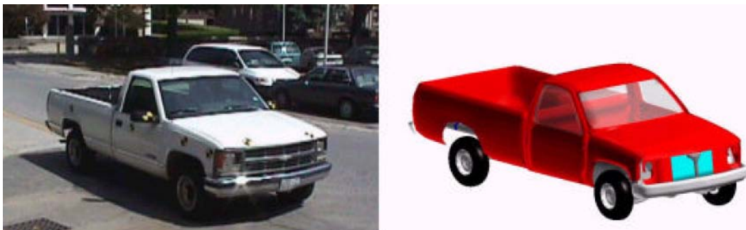
Figure C8-1. View of a 1995 C2500 pickup truck (a) actual vehicle and (b) finite element model of the vehicle.
