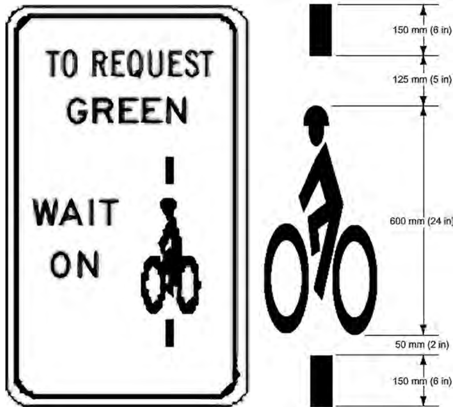
Standard stencil and signage show cyclists how to get a green light Source: MUTCD
