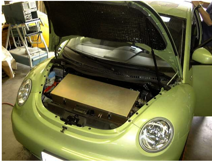
Figure 7. AC150 Gen-2 drivetrain with bi-directional grid power capability installed in Beetle EV
