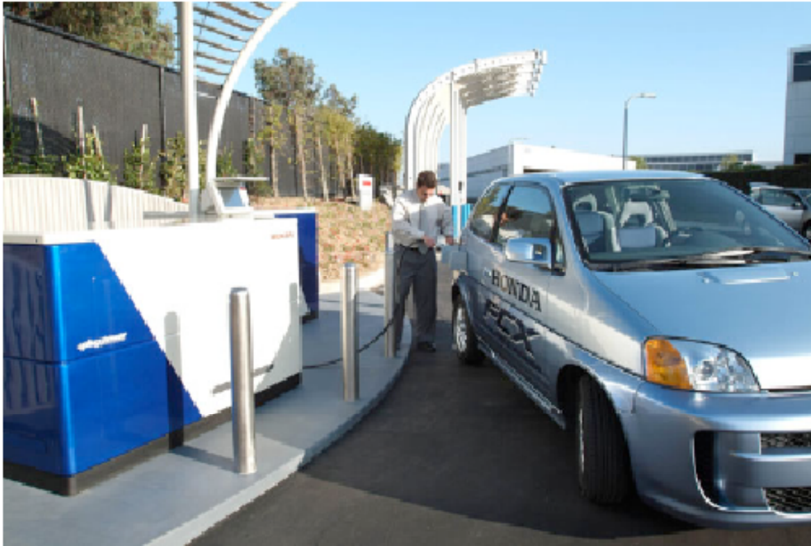
Figure 5-3: Demonstration of the Honda/Plug Power H 2 E-Station
