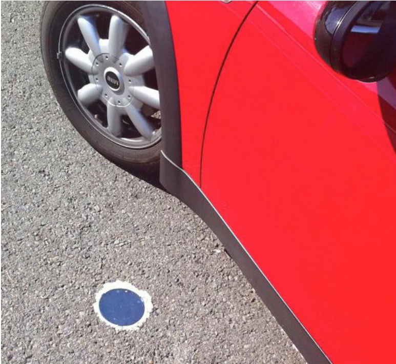
Figure E-1. LA Express Park™ In-Ground Parking Sensor
