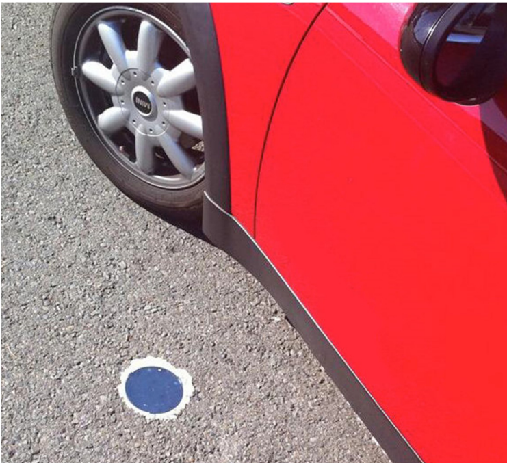
Figure 5-8. LA Express Park™ In-Ground Parking Sensor
