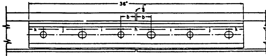
FIGURE 2 - JOINT BAR SHOWING ROUND AND OVAL BOLT HOLES
