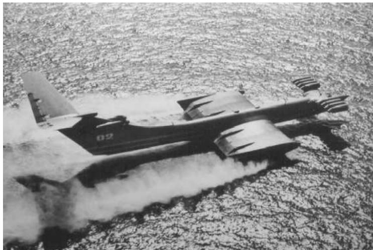
Figure 7: Wings in ground effect: KM Caspian Sea Monster (10)
