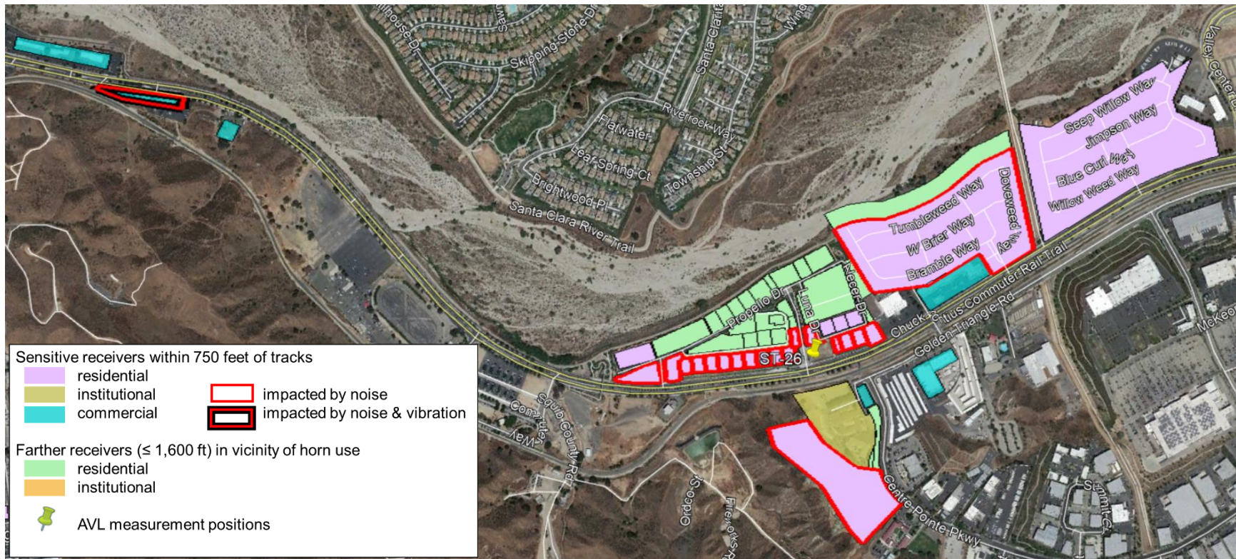
Figure 3.10-7: Construction Noise and Vibration Impacts in Vicinity of Canyon Siding Extension in the City of Santa Clarita
