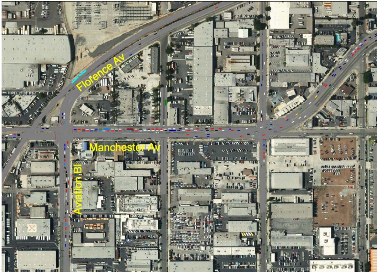
Figure 5-1. Future 2030 with LRT and Potential Mitigation Traffic Queuing Conditions Snapshot at Aviation Boulevard/Manchester Avenue Intersection in A.M. Peak Hour
