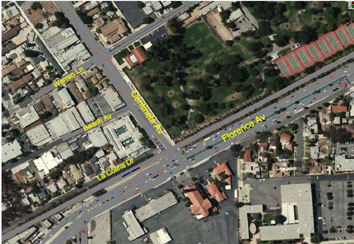
Figure 5-3. Future 2030 with LRT and Potential Mitigations Traffic Queuing Conditions Snapshot at Florence Avenue/Centinela Avenue Intersection in A.M. Peak Hour
