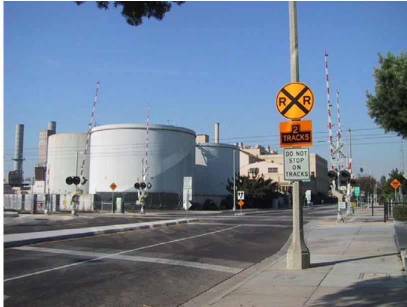
Figure 4-54. At-Grade LRT Crossing with Safety Features
