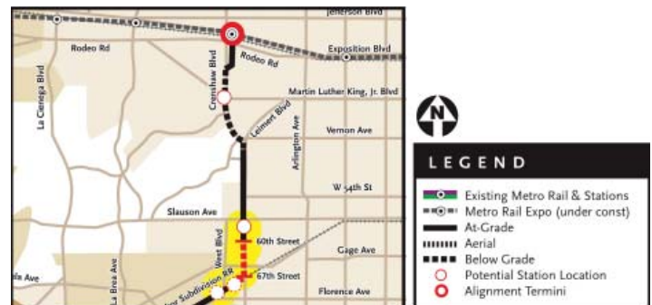
To eliminate the visual effects of an elevated LRT structure within the median of Crenshaw Boulevard, Design Option 4 considers below grade alignment from 60th street to Victoria Avenue.
