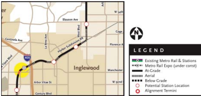
LRT Design Option 2 addresses whether an elevated crossing above Manchester Avenue is necessary to preserve efficient traffic flow during LRT operations.
