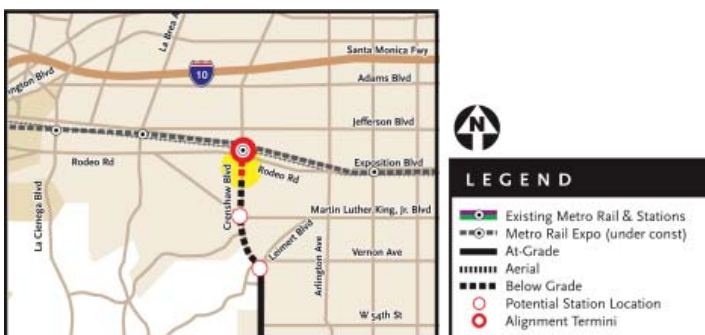
To reduce potential traffic conflicts at Exposition and Crenshaw and to avoid right-of-way conflicts with a proposed development along Crenshaw Boulevard between Rodeo Road and Coliseum Street, LRT Design Option 6 considers a below grade alignment along Crenshaw Boulevard between Exposition and 39th Street.
