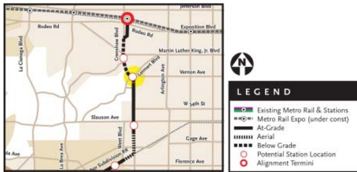
LRT Design Option 5 considers the feasibility of maintaining two stations in close proximity at Crenshaw/King and at Crenshaw/Vernon. The Crenshaw/Vernon station is the optional station.
