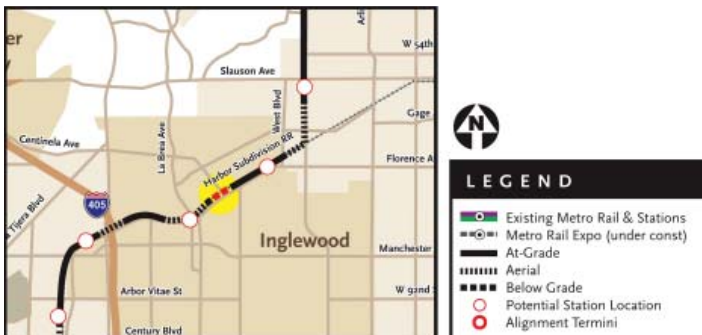
LRT Design Option 3 considers the effects of creating a grade separation at the Harbor Subdivision and Centinela Avenue. This crossing is at grade in the Base LRT Alternative, however, there are adjacent land uses such as a nearby school, and park that generate pedestrian traffic that would have to cross the LRT line.
