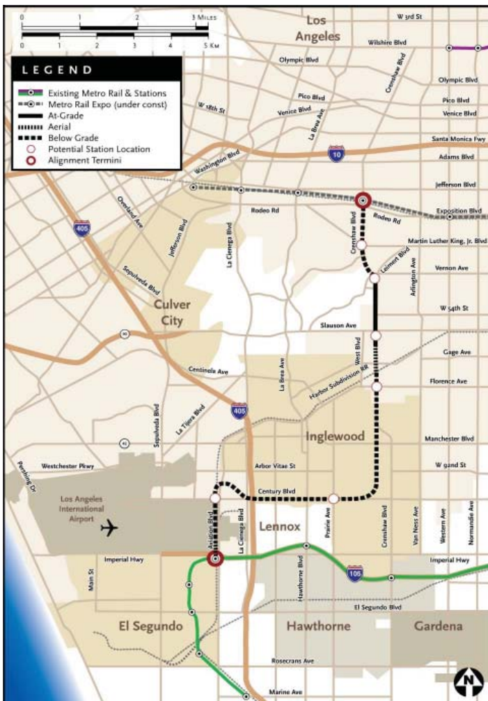
A Crenshaw/Century Boulevard alignment was eliminated since it would require tunneling under residences, abandoned oil wells and across earthquake faults, raising the cost significantly.
