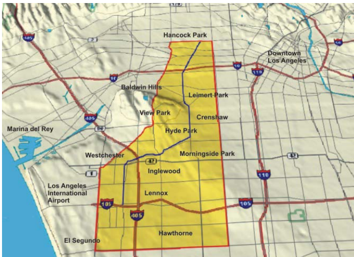
The Baldwin Hills are a significant topographic constraint in the Crenshaw Corridor. The feature limits the continuity of the transportation network in both north-south and east-west directions increasing the importance of efficient traffic flow along Crenshaw Boulevard.
