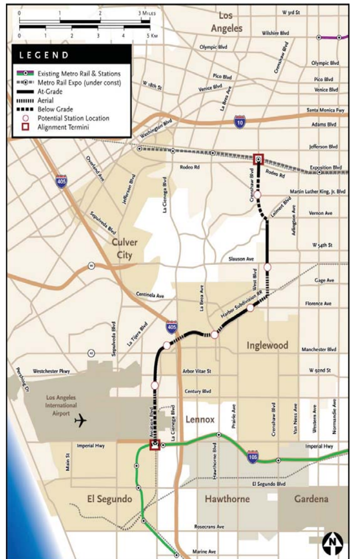
Base LRT Alignment. The Base light rail route is approximately 8.5 miles in length. It extends from the Exposition Light Rail line to the Green Line. This baseline option includes at grade, below grade and elevated sections as shown above.
