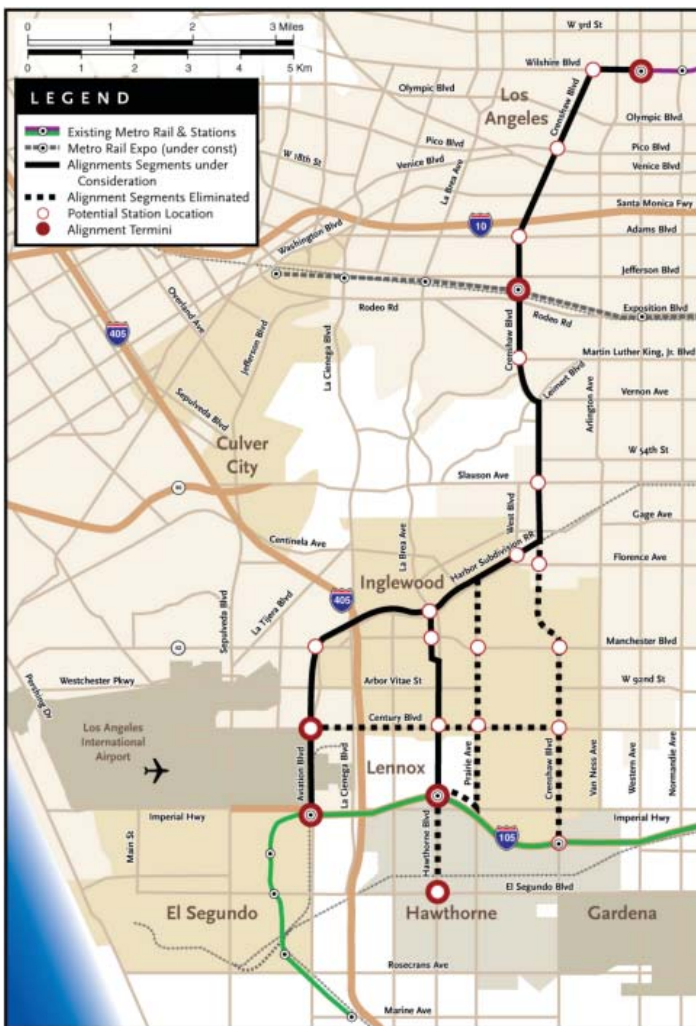
Alignments Eliminated in Initial Study Screening. The dotted lines indicate the alignments eliminated from further study. Options were eliminated due to physical and engineering constraints, lack of community acceptance, and potential adverse environmental effects.
