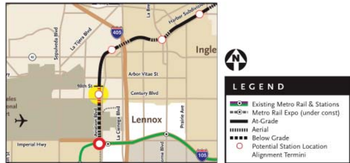
Design Option 1 considers whether the proposed LRT station at Aviation/Century should be elevated and be located closer to Century Boulevard.
