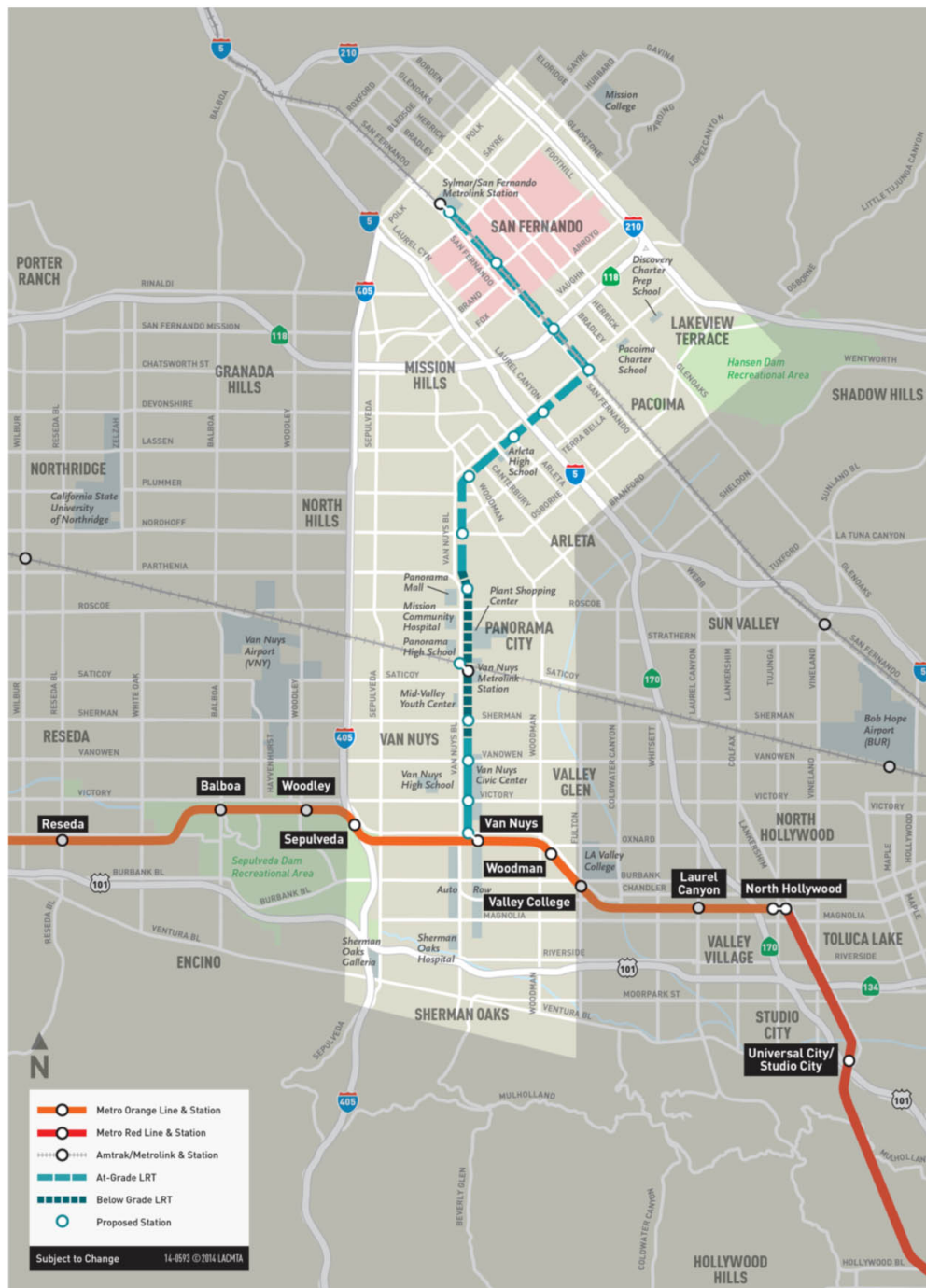
Figure 1-4 – Alternative 4 East San Fernando Valley Transit Corridor Median Running Light Rail Transit (LRT)
