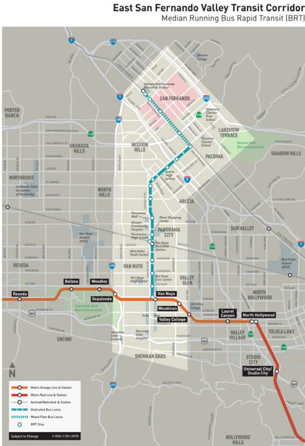
Figure 1-3: Build Alternative 2 – Median-Running BRT Alternative
