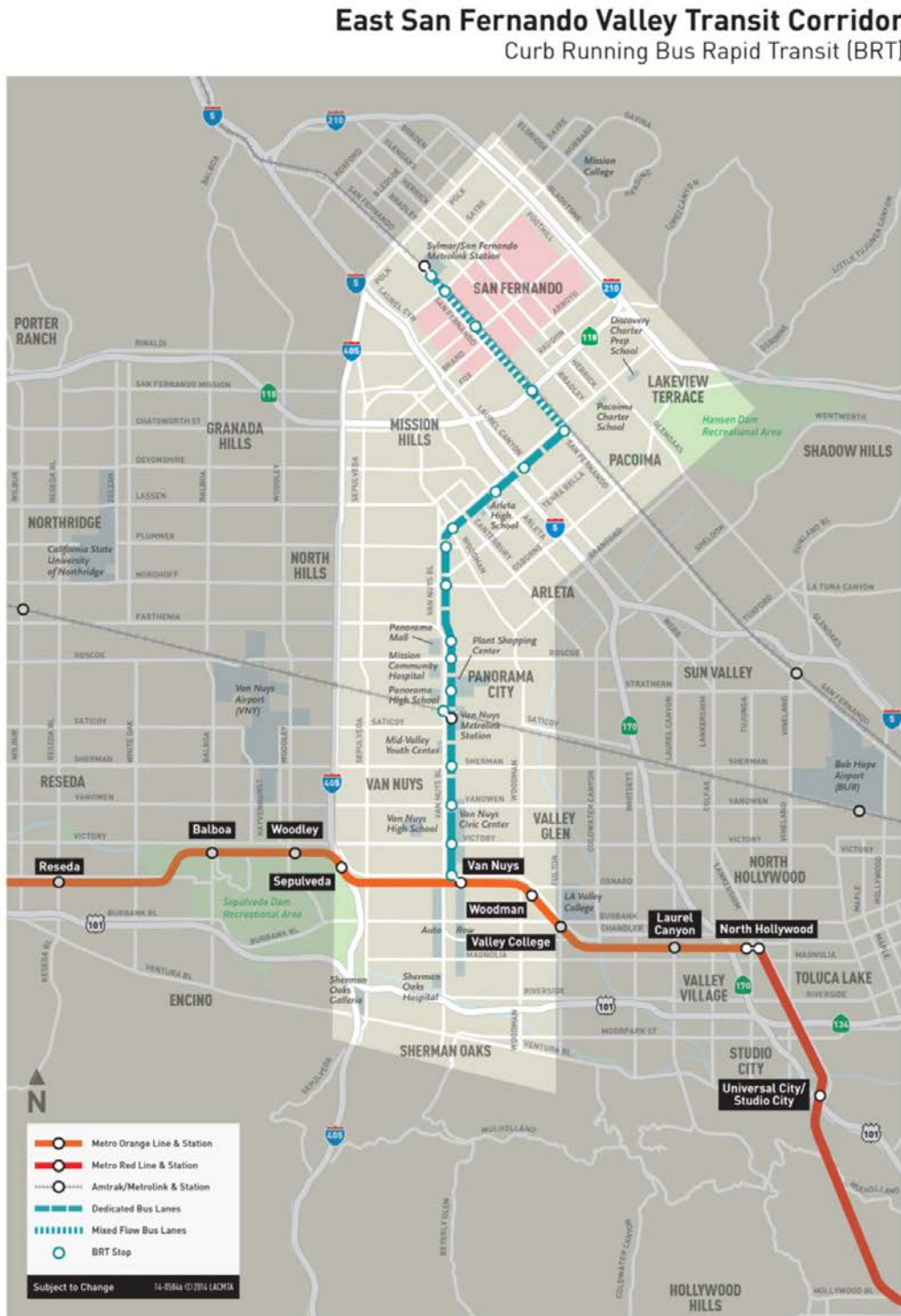
Figure 1-2: Build Alternative 1 – Curb-Running BRT Alternative
