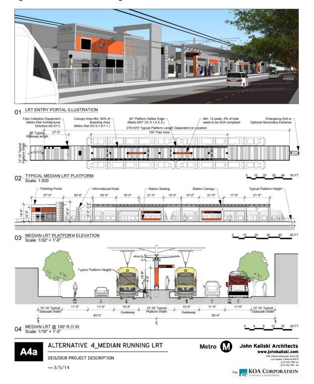
Figure 1-13: Architectural Rendering for LRT Alternative
