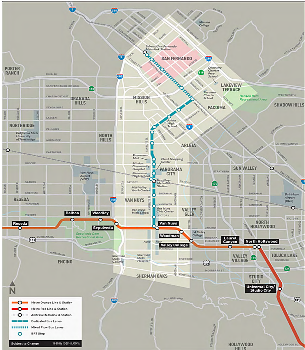
Figure 2-3: BRT Alternatives – Alternative 1: Curb-Running BRT
