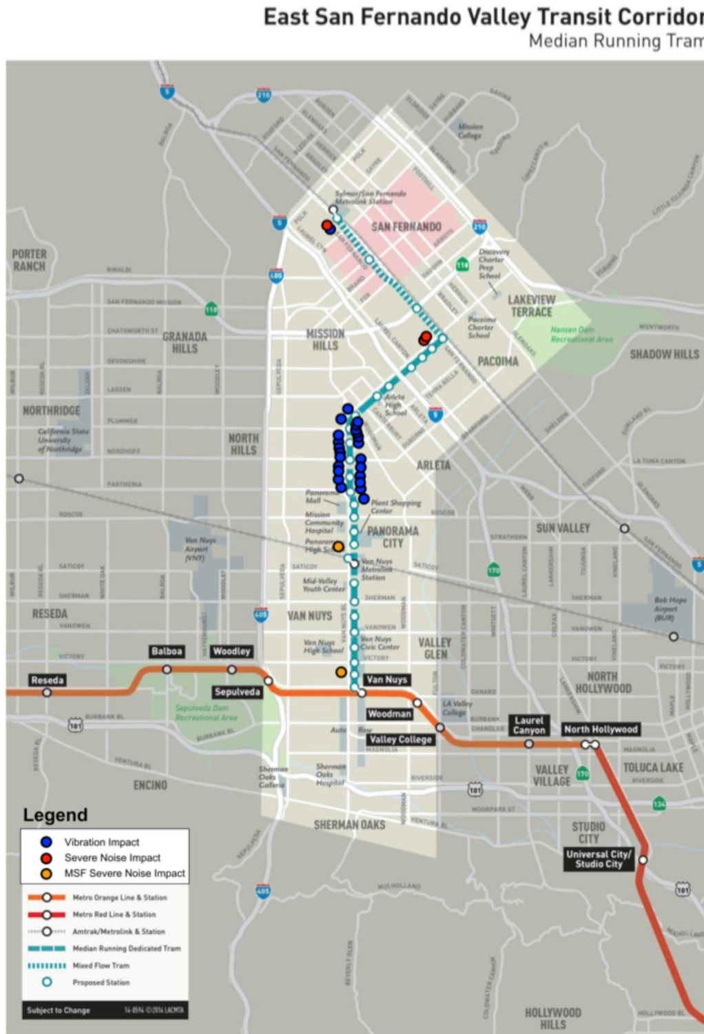
Figure 4.8-3: Map of Predicted Operational Impacts for Low-Floor LRT/Tram Alternative
