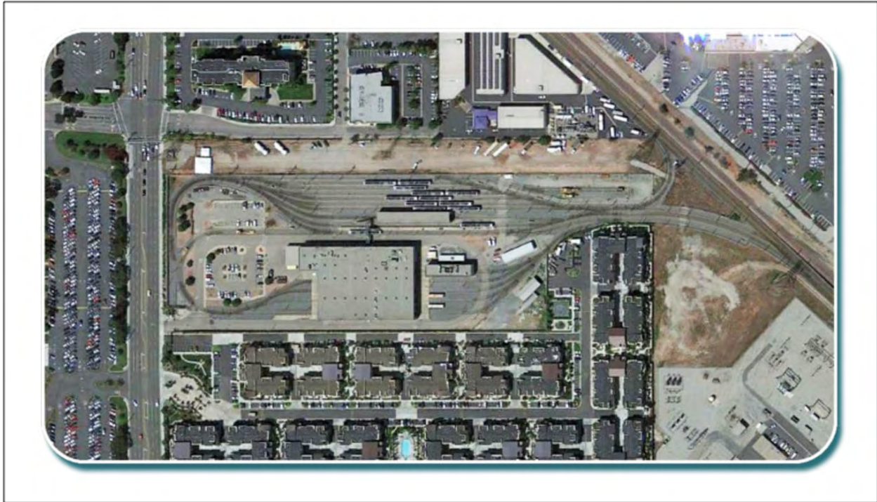
Figure 2-11: Typical MSF Facility for Tram/LRT
