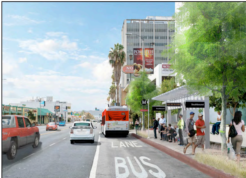
Figure 4.5-11: Illustrative View of Curb-Running BRT Alternative
