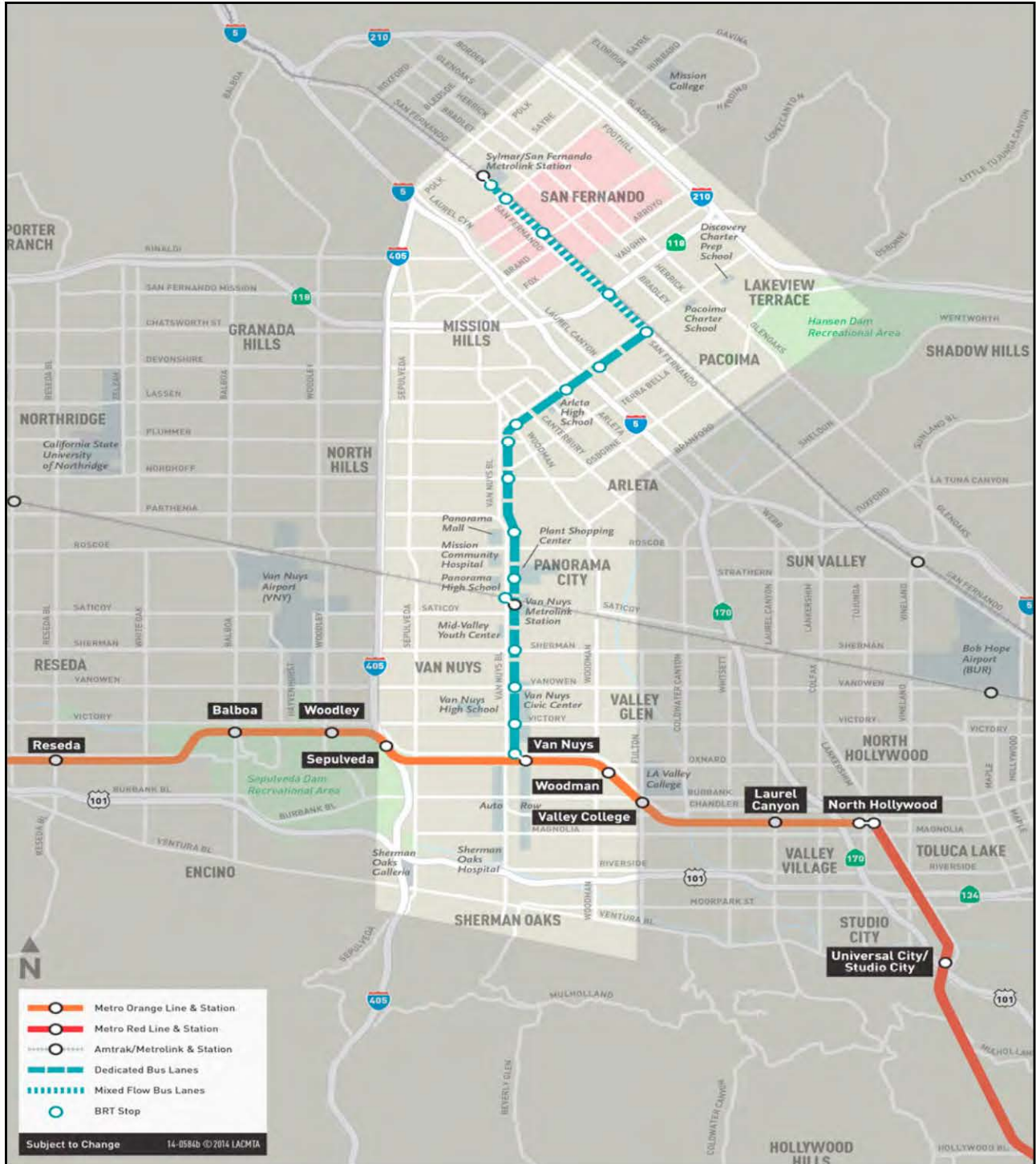
Figure ES-5: Alternative 2 – Median-running BRT
