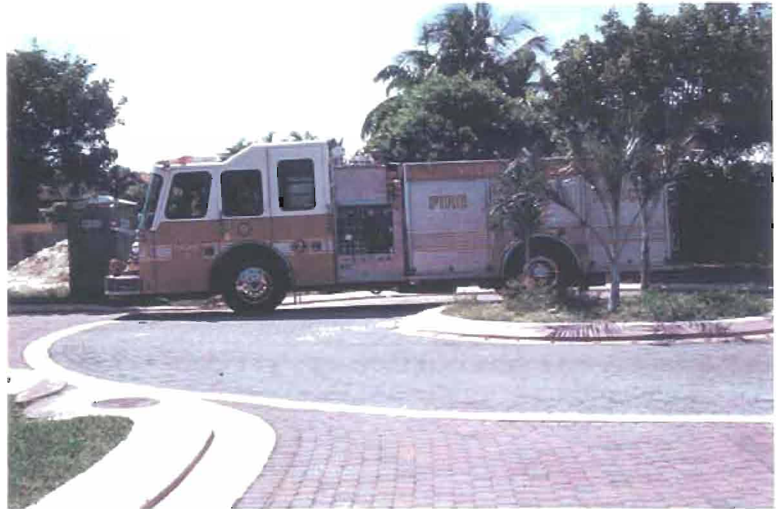
Fire truck successfully negotiating a typical mini circle on a non-framework street.
