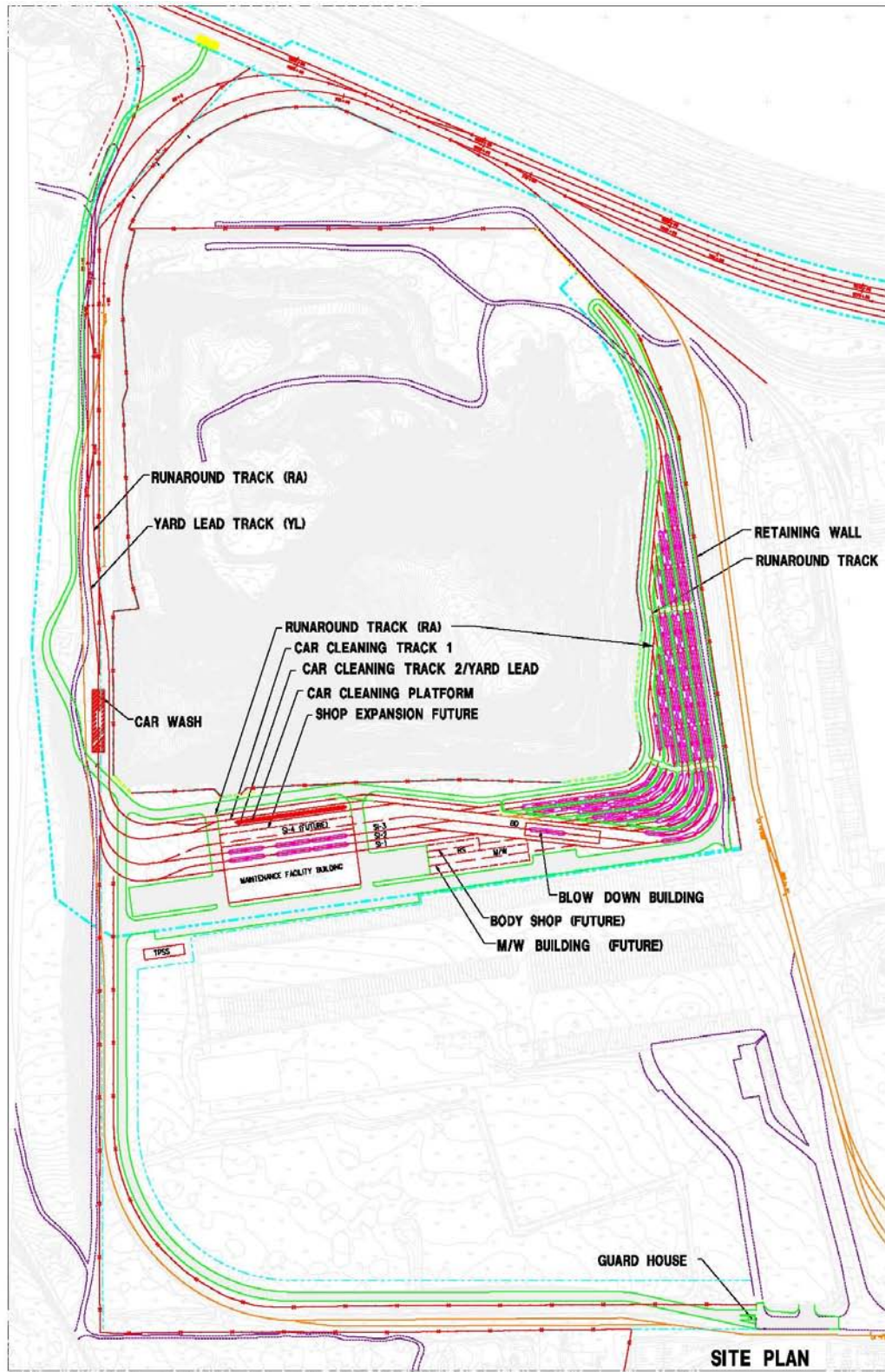
Figure 2-49: Site Plan: Maintenance and Operations Facility, Irwindale
