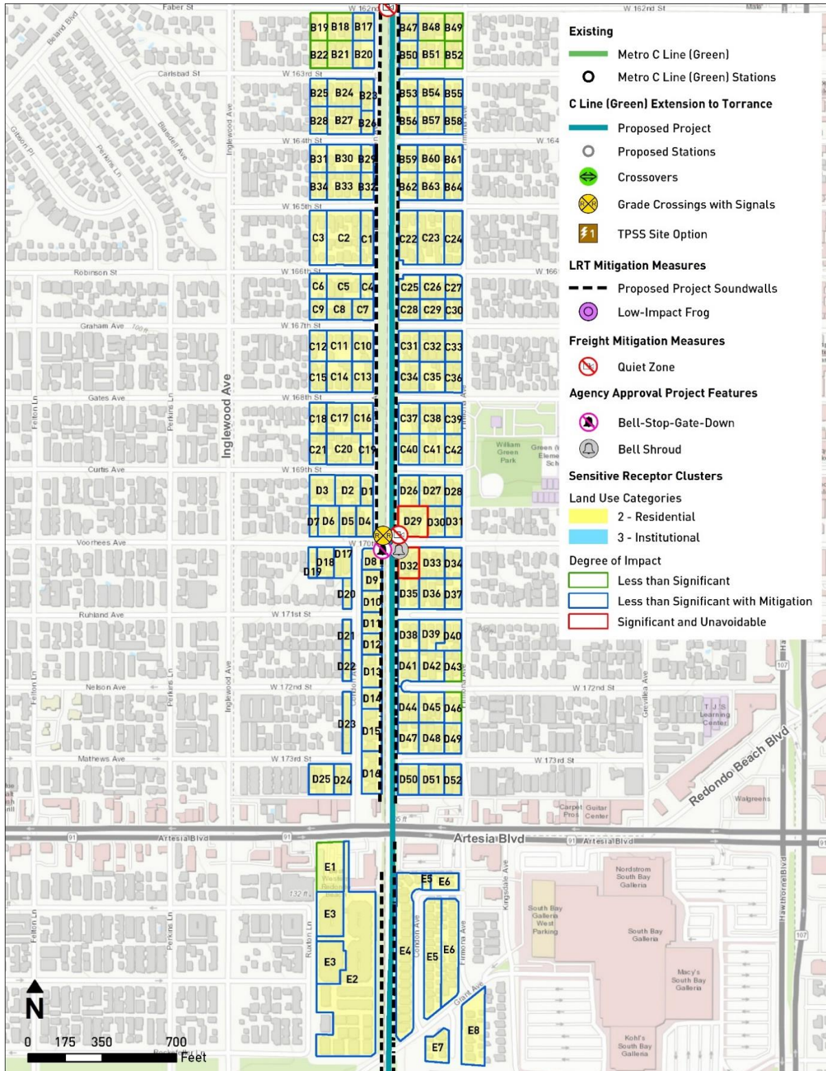
Figure 3.6-22. Proposed Project – Combined Light Rail and Freight Relocation Mitigated Noise Impacts (2 of 4)
