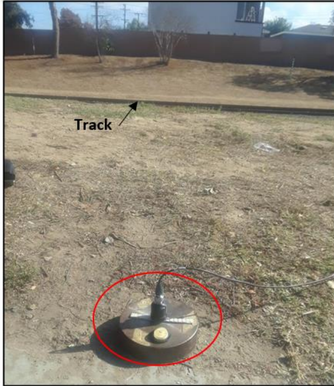
Figure 3.6-10 Vibration Measurement Set-ups
