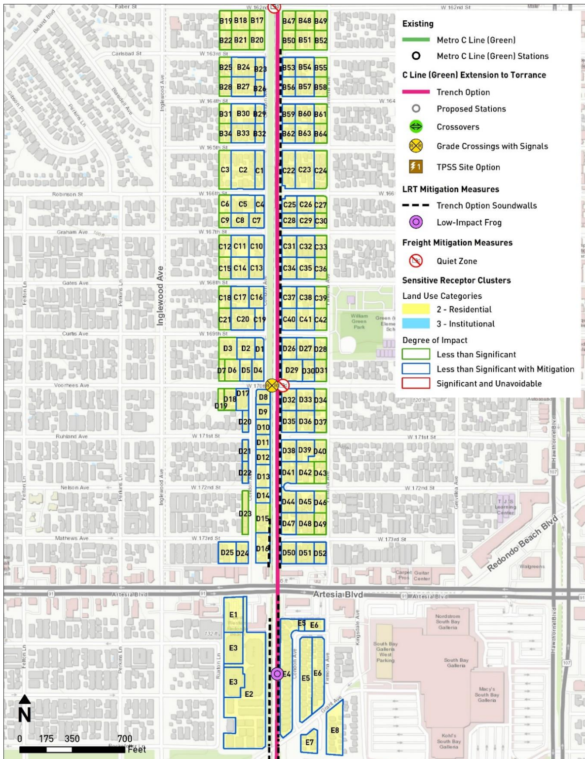
Figure 3.6-26. Trench Option – Combined Light Rail and Relocated Freight Mitigated Noise Impacts (2 of 3)
