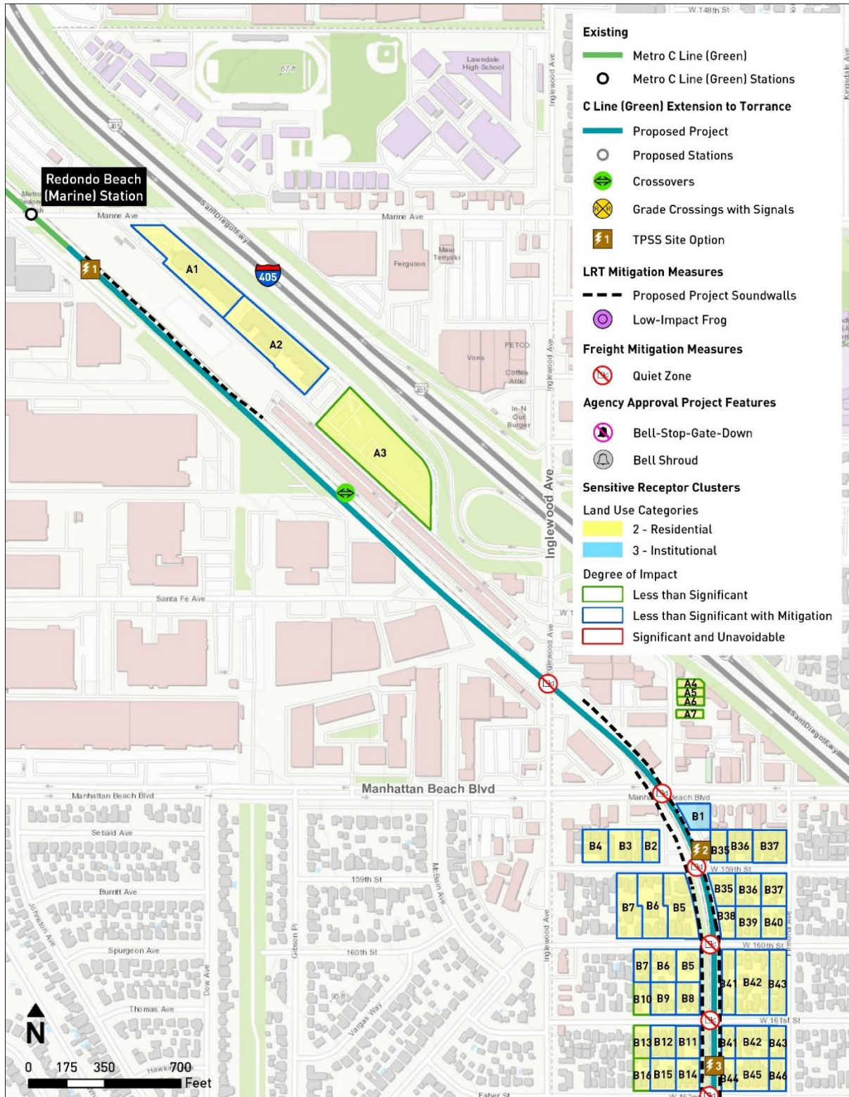
Figure 3.6-21. Proposed Project - Combined Light Rail and Freight Relocation Mitigated Noise Impacts (1 of 4)
