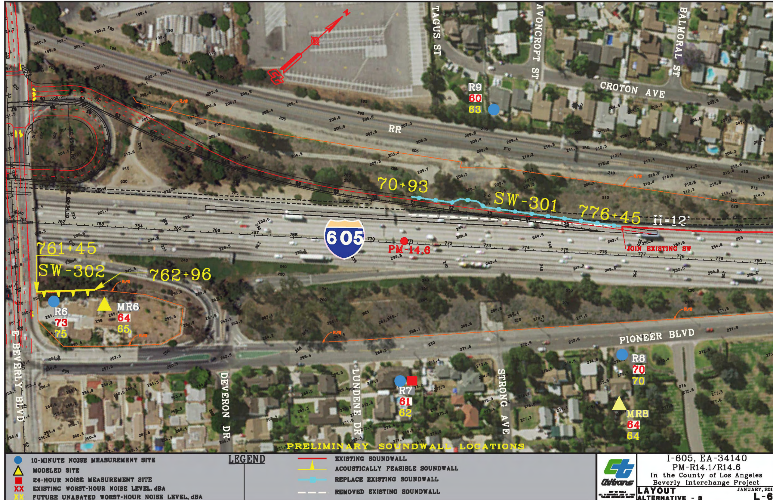
Figure 19 – Preliminary Soundwall Locations
