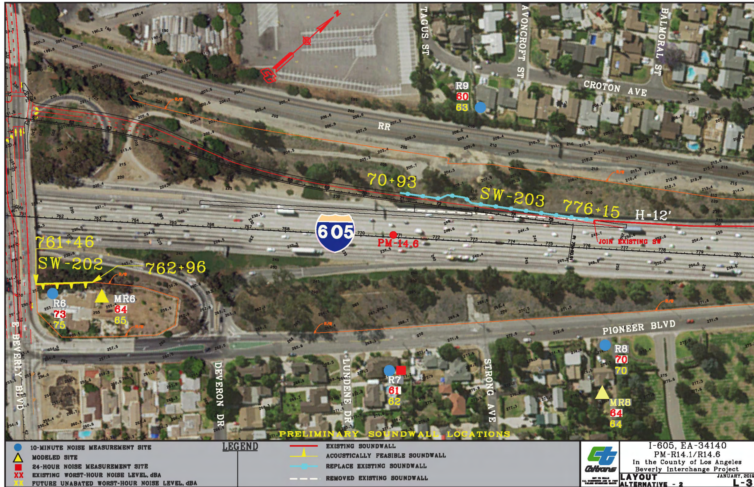
Figure 16 – Preliminary Soundwall Locations
