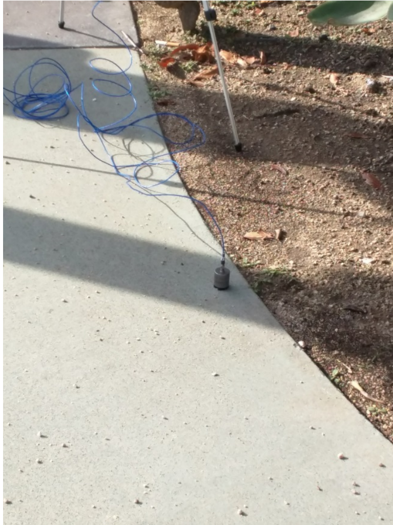
Figure B-19. Monitoring Location 3 Vibration Meter Setup, #1
