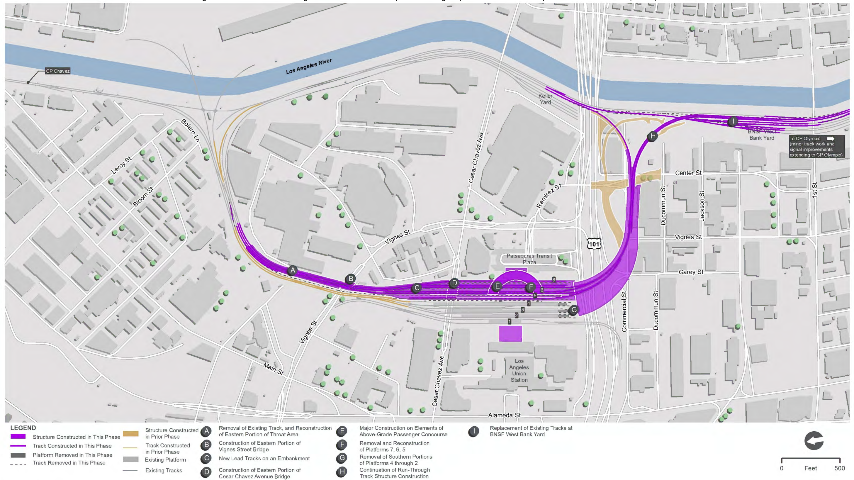
Figure 1-2. Above-Grade Passenger Concourse with New Expanded Passageway Construction Scenario (Phase II Construction Steps 7-12)
