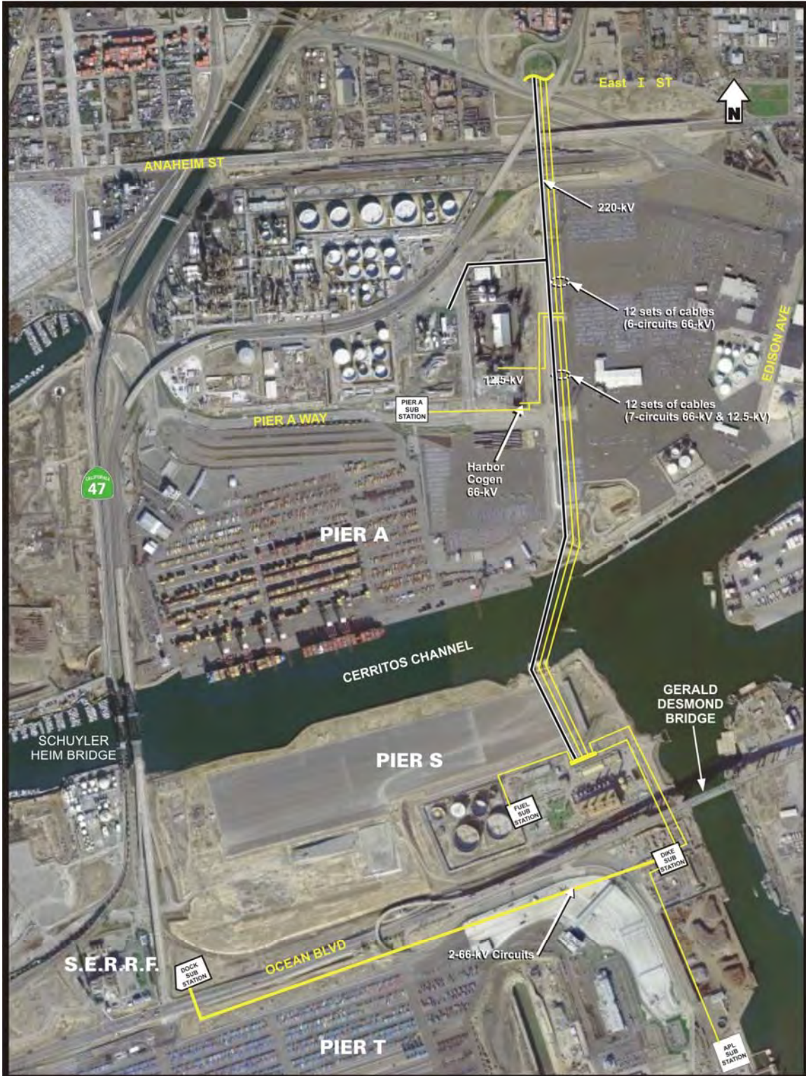
Figure 2 Existing Electrical Placement
