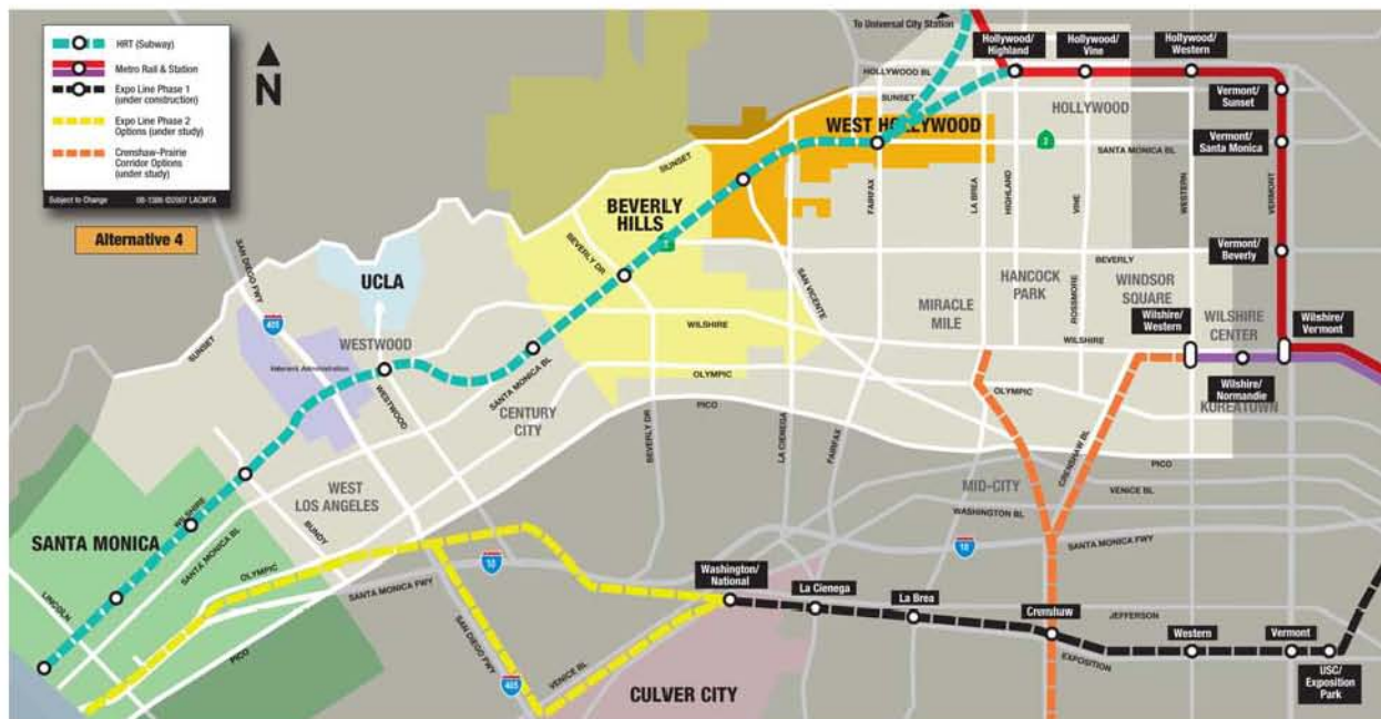
Figure 2-14. Alternative 4 – Santa Monica Boulevard Alignment HRT Subway
