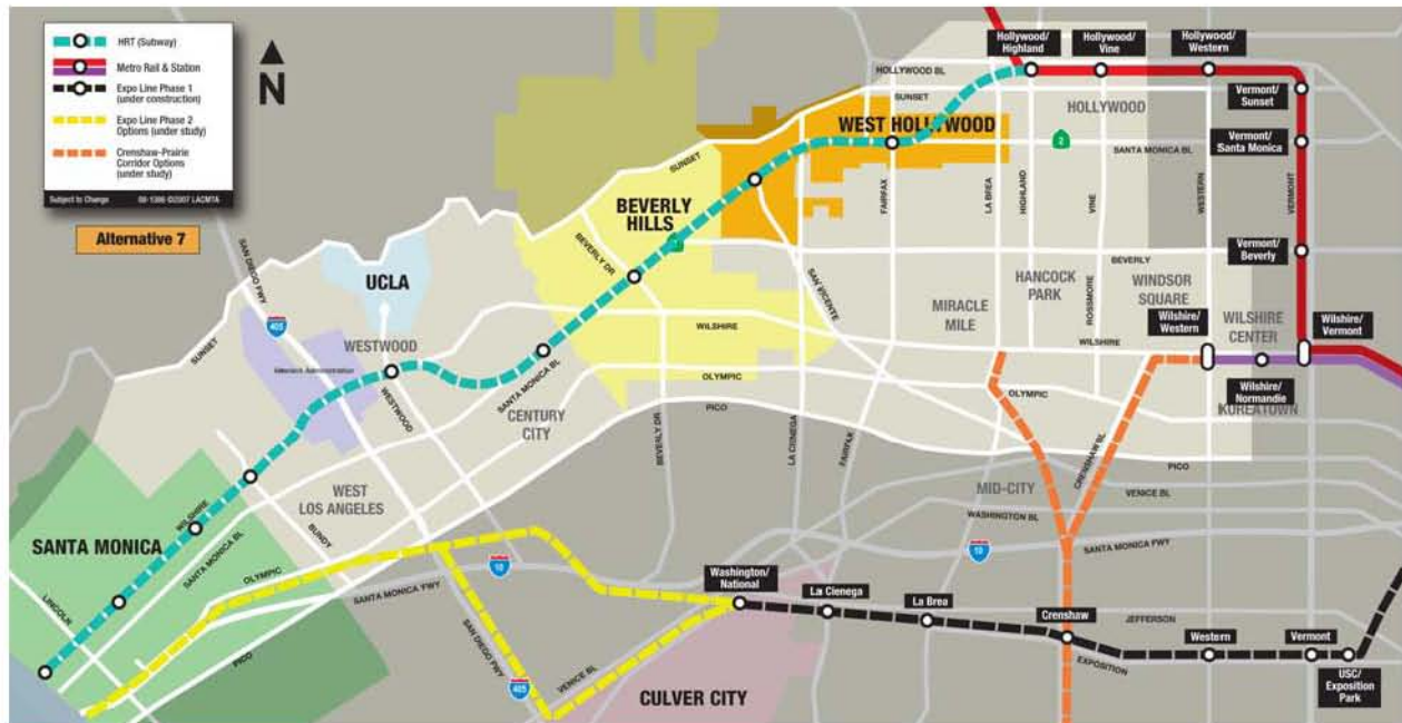
Figure 2-16. Alternative 7 – Santa Monica Boulevard Alignment HRT Subway with Hollywood/Highland Red Line Connection/Galaxy North
