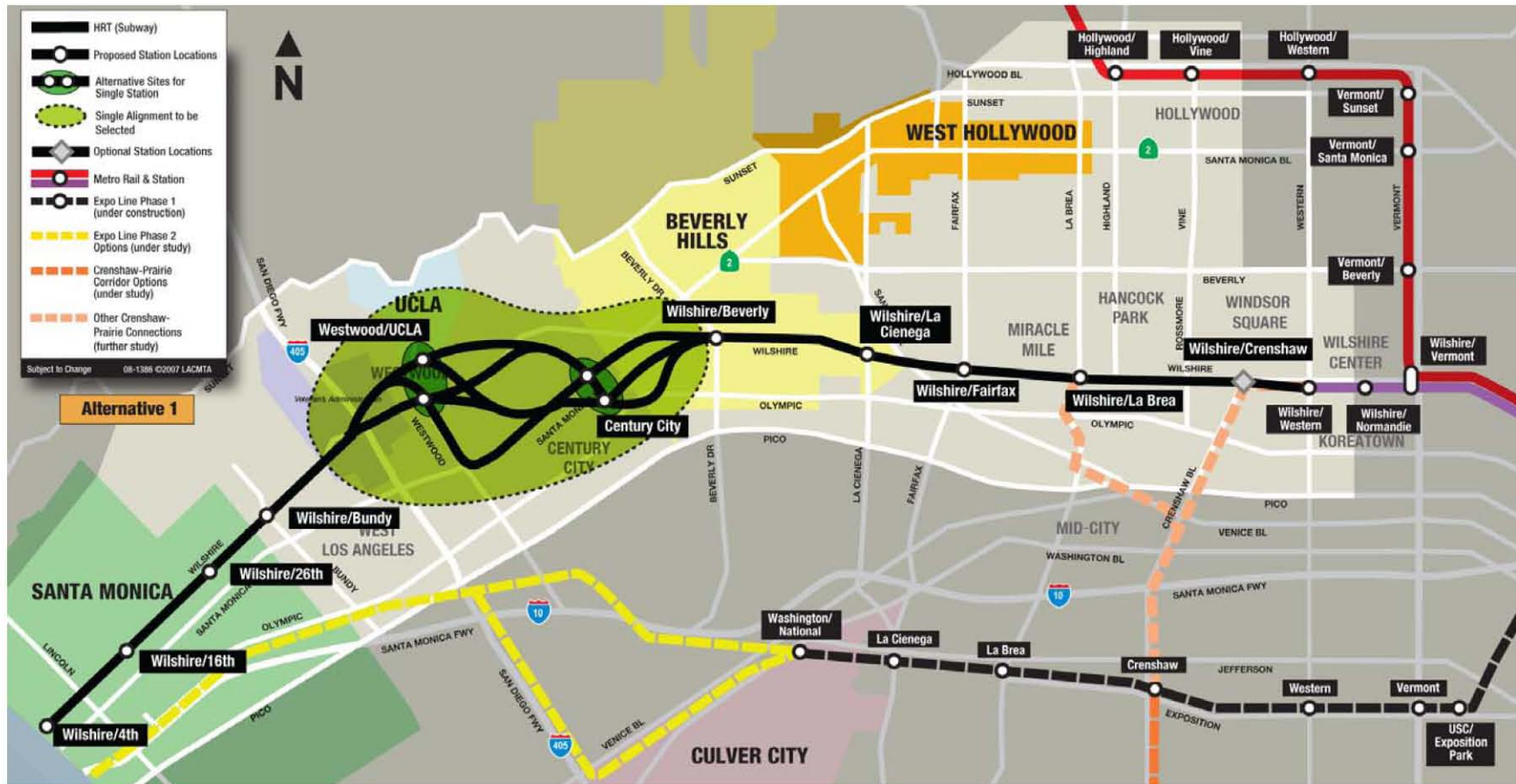
Figure 2-40. Alternative 1 - Wilshire Boulevard Alignment HRT Subway
