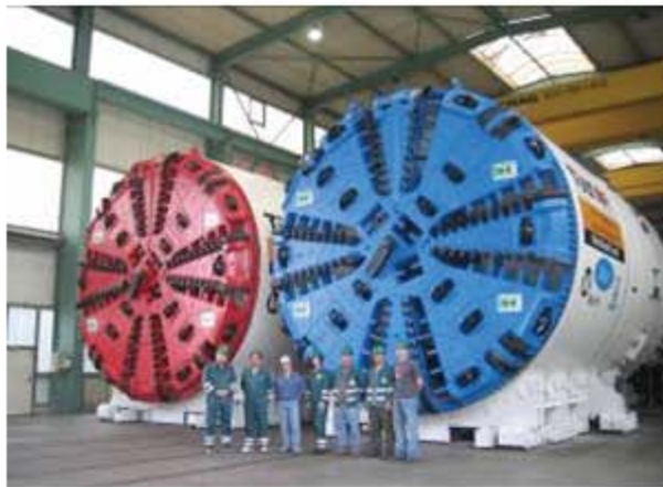
Figure S-42 Tunnel Boring Machines used for Gold Line Eastside Extension
