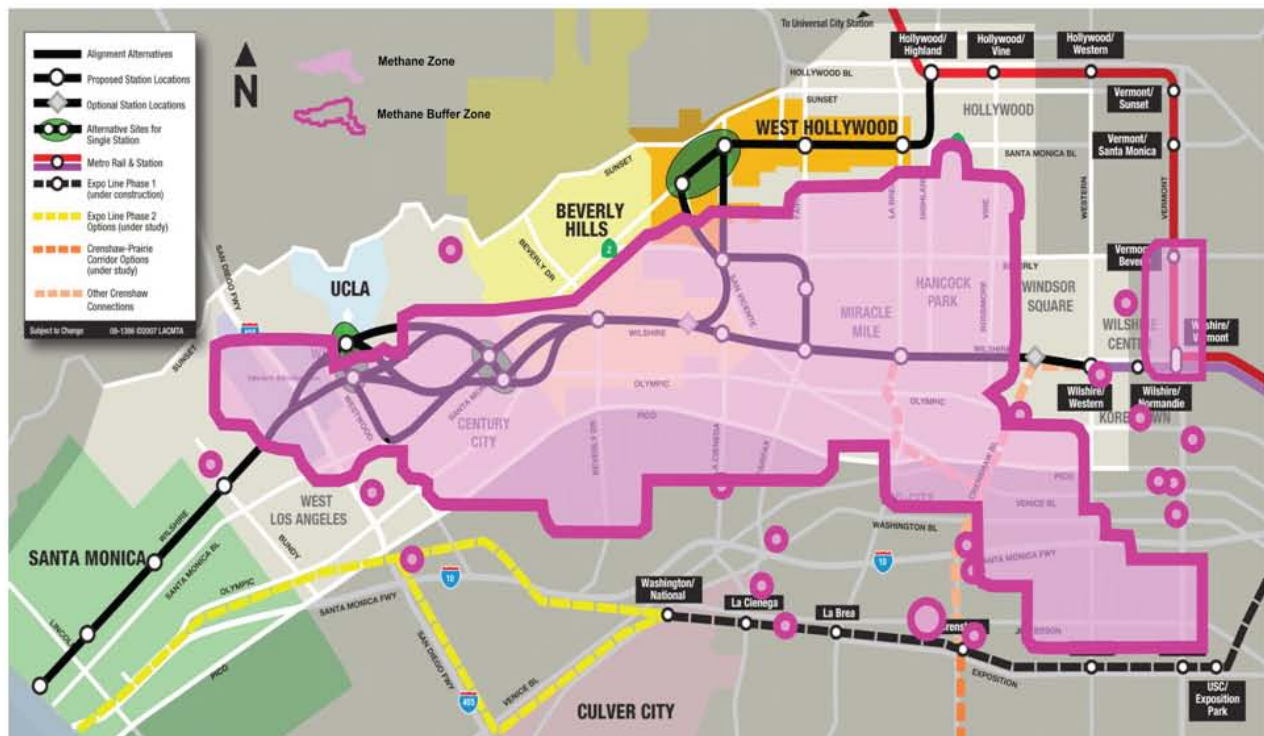
Figure S-43 Study Alignments with Methane Risk Zone and Methane Buffer Zone
