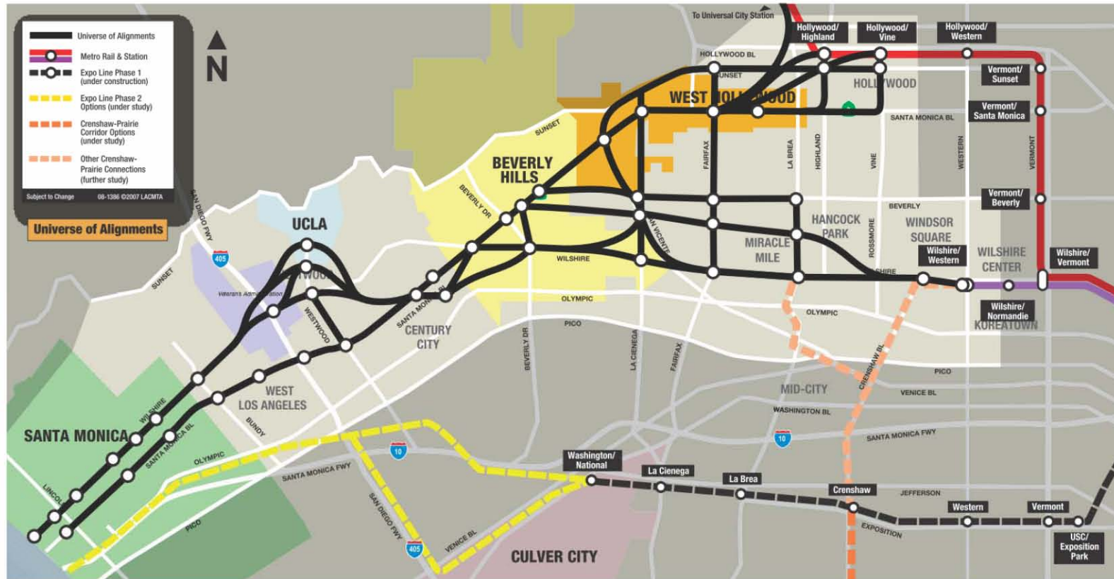
Figure 2-6. Universe of Alignments and Station Alternatives
