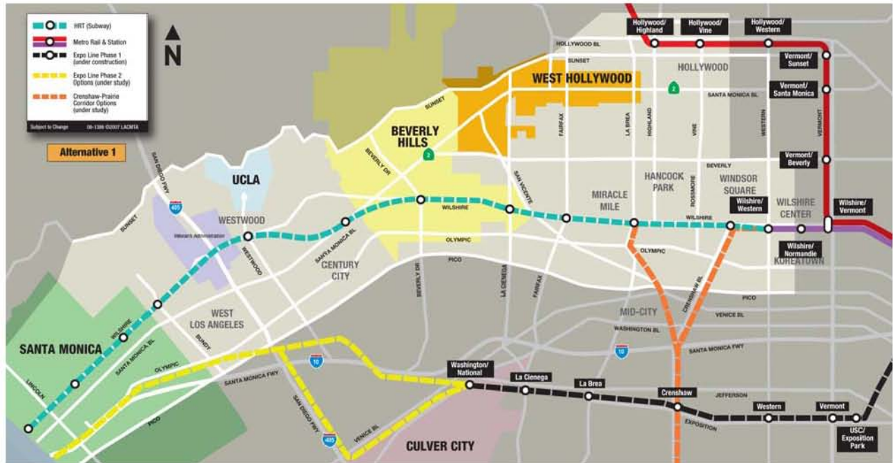
Figure 2-10. Alternative 1 – Wilshire Boulevard Alignment HRT Subway
