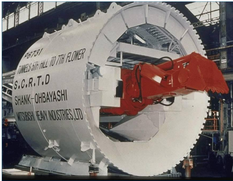
Figure 2.2-11: Open-Face of Digger Shield used to Construct Metro Red Line Contract A146 Tunnels
