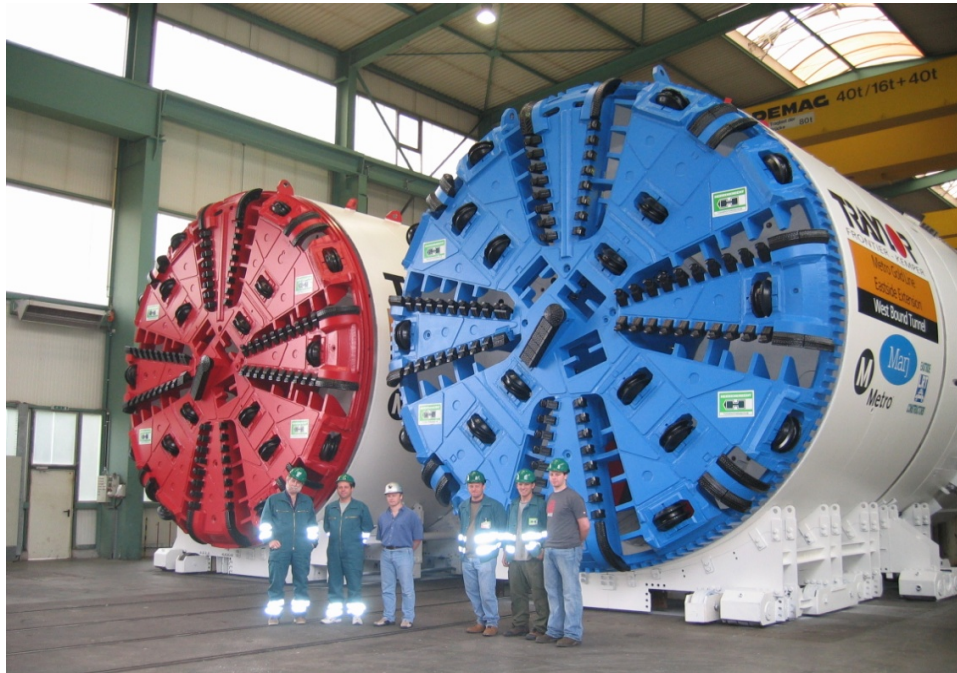
Figure 4-15: EPBMs Used for Constructing Los Angeles Eastside LRT Tunnels
