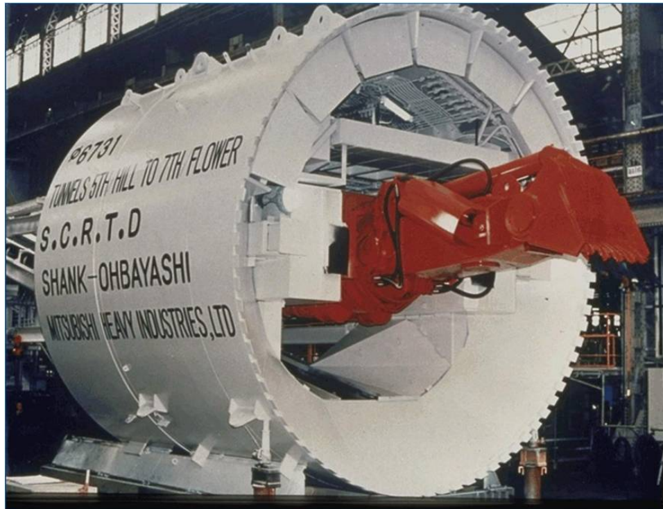
Figure 4-1: Digger Shield Used to Construct Metro Red Line Contract A146 Tunnels
