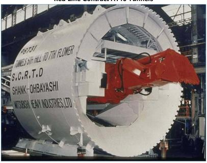
Figure 2.2-11: Open-Face of Digger Shield used to Construct Metro
