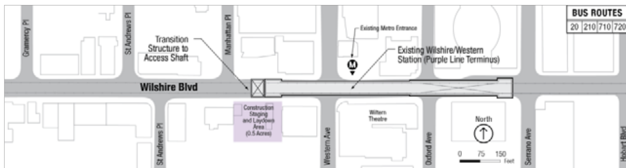
Figure 4-13: Wilshire/Western Station—Transitional Structure and Construction Staging and Laydown—South of Wilshire
