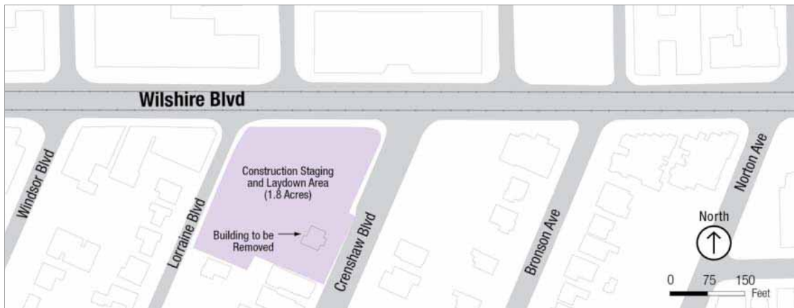
Figure 4-14: Wilshire/Crenshaw Construction Staging and Laydown
