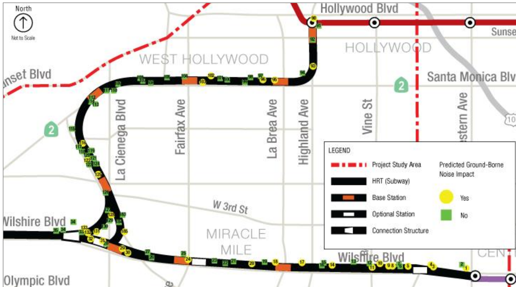
Figure 5-5. Vibration Sensitive Locations—Barrington Ave to 2 nd Street
