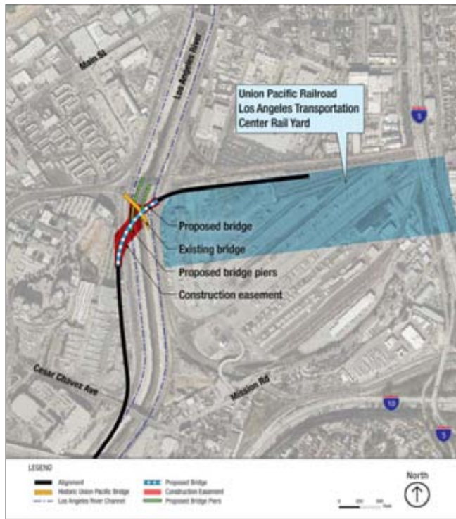
Figure 2-14. UP Railroad Rail Bridge
