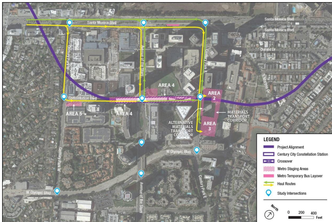
Figure 3-5. Proposed Construction Truck Haul Routes
