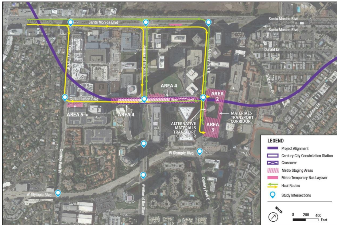
Figure 3-5. Proposed Construction Truck Haul Routes
