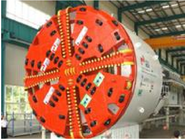
Figure 4-23. Pressurized-Face Tunnel Boring Machine
