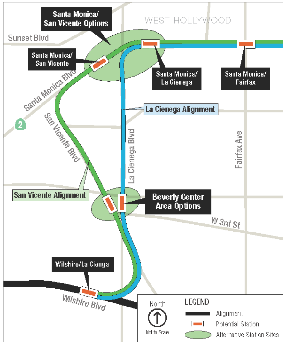
Figure 4-31: West Hollywood Alignment and Station Options
